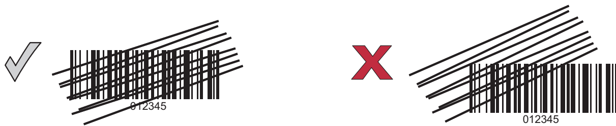
Figure 2-3 Acceptable and Incorrect Multi-Line Aiming
